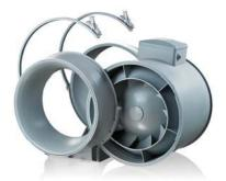
spigots by means of special clamps with latches. This makes the fan maintenance fast and easy. The fan maintenance does not require total disassembling. Just pull out the central block from the casing and perform required servicing. All the models may be equipped with a regulated timer with turn-off delay adjustable from 2 to 30 min.
